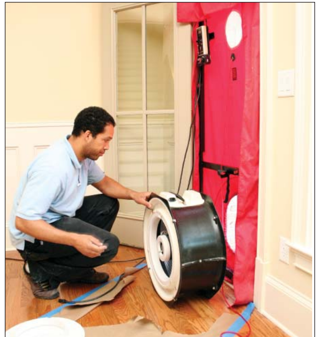
Blower door diagnostics indicate the level of "tightness" of a building. This helps determine air leakage of the building and pinpoint areas for sealing.
