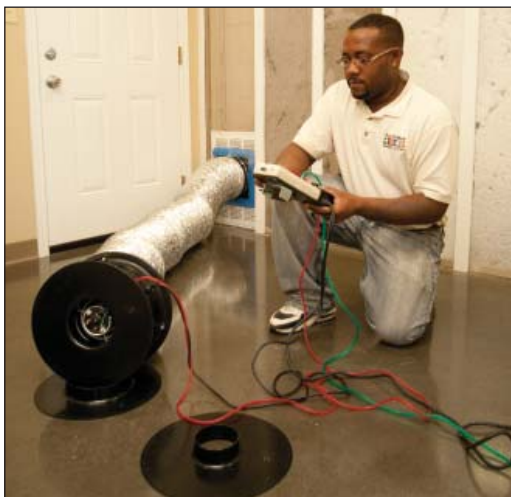
This technician is performing a duct leakage test that ensures the integrity of the duct system.
